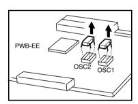
6 Install the Oscillator Chip supplied into the OSC1 socket as shown on the illustration
